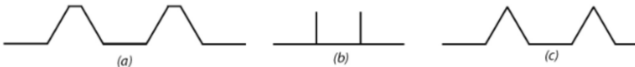
Different geometry types of riblets: (a) trapezoidal, (b) bladed, (c) triangular.
